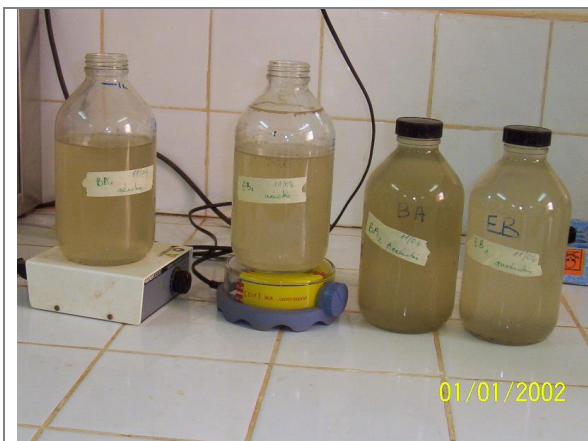
Photo V. 4: Essai de Nitrification/dénitrification
