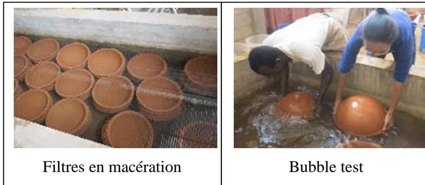
**Figure 9: Le bubble test**
