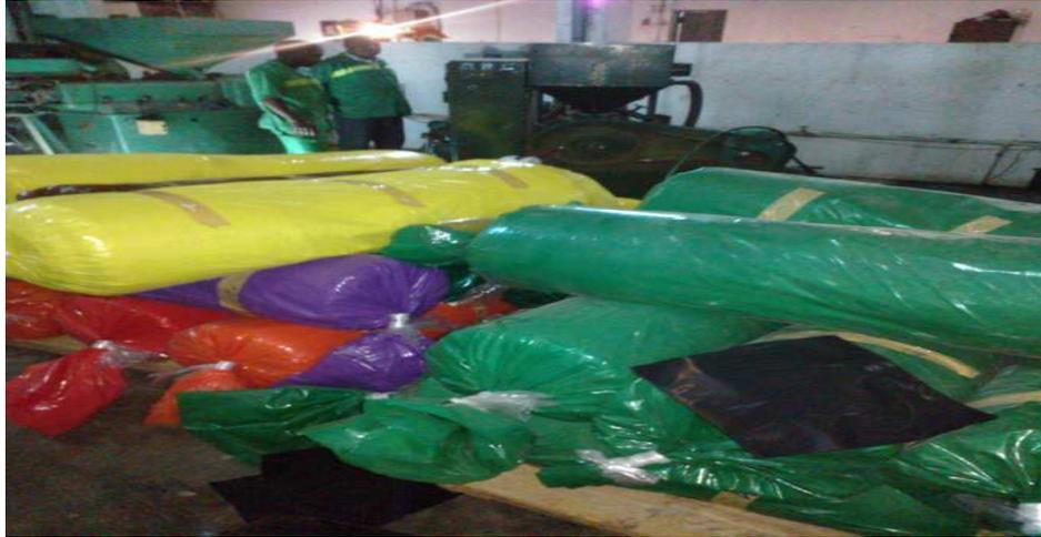
*Photo 5: gaines plastiques (55mm × 25µm).*
