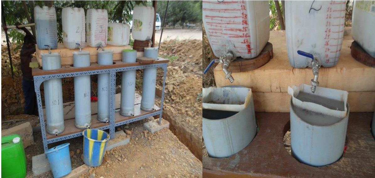
Figure 3-1. Vermifiltration experiment at 1000 \text{ L.m}^{-2}.\text{d}^{-1} at a continuous flow at 2iE campus in Ouagadougou, Burkina Faso
