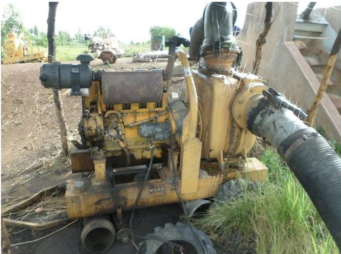
**Figure 13: Moto pompe thermique station SP50**
