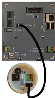
A maximum of four BMVs can be connected directly to the Color Control.
