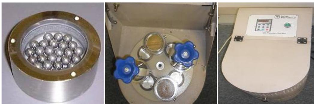
Figure 3 Stainless steel bowl with stainless steel balls (left), holder (middle), HEBM (right).
