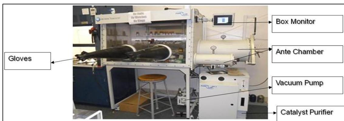
Figure 5 Nitrogen filled Glove box
