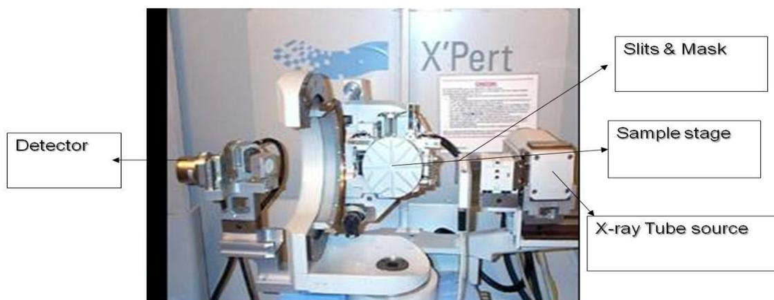
Figure 8 X-ray Diffraction with vertical goniometry ( $\theta$ - $2\theta$ )
