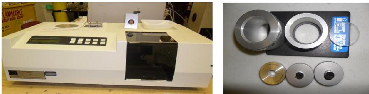
Figure 6 FT-IR instrument (left), KBr die set and KBR window (right).
