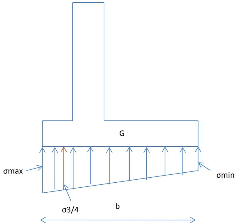
$$\sigma_{max} = \frac{N}{S} \times \left(1 + \frac{6 \times |e_{/G}|}{b}\right) = \frac{239,375}{3,35 \times 1} \left(1 + \frac{6 \times 0,15}{3,35}\right) = 90,65 \text{ KN/m}^2$$
