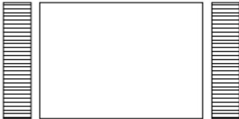
La contrainte horizontale :  $\sigma = k \times q = 0,33 \times 10 = 3,33 \text{ kN/m}^2$
