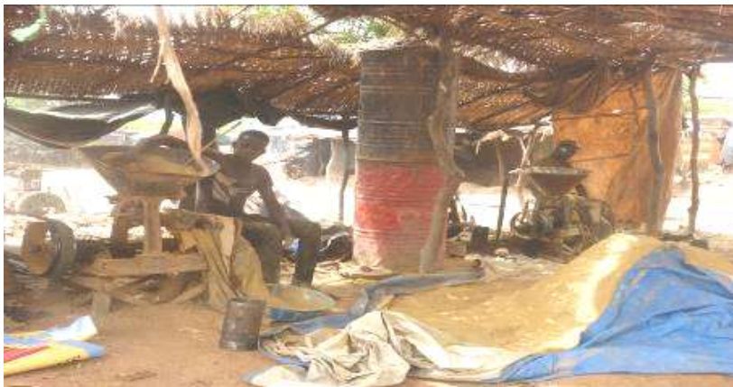
Figure 6: Broyage du minerai
