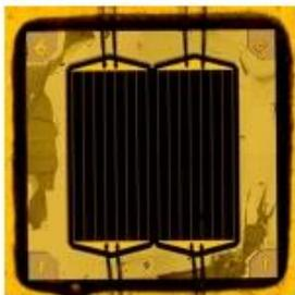
Figure 10: cellule multi-jonction
