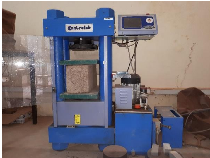
Photo 1 : Essai de compression parpaing
