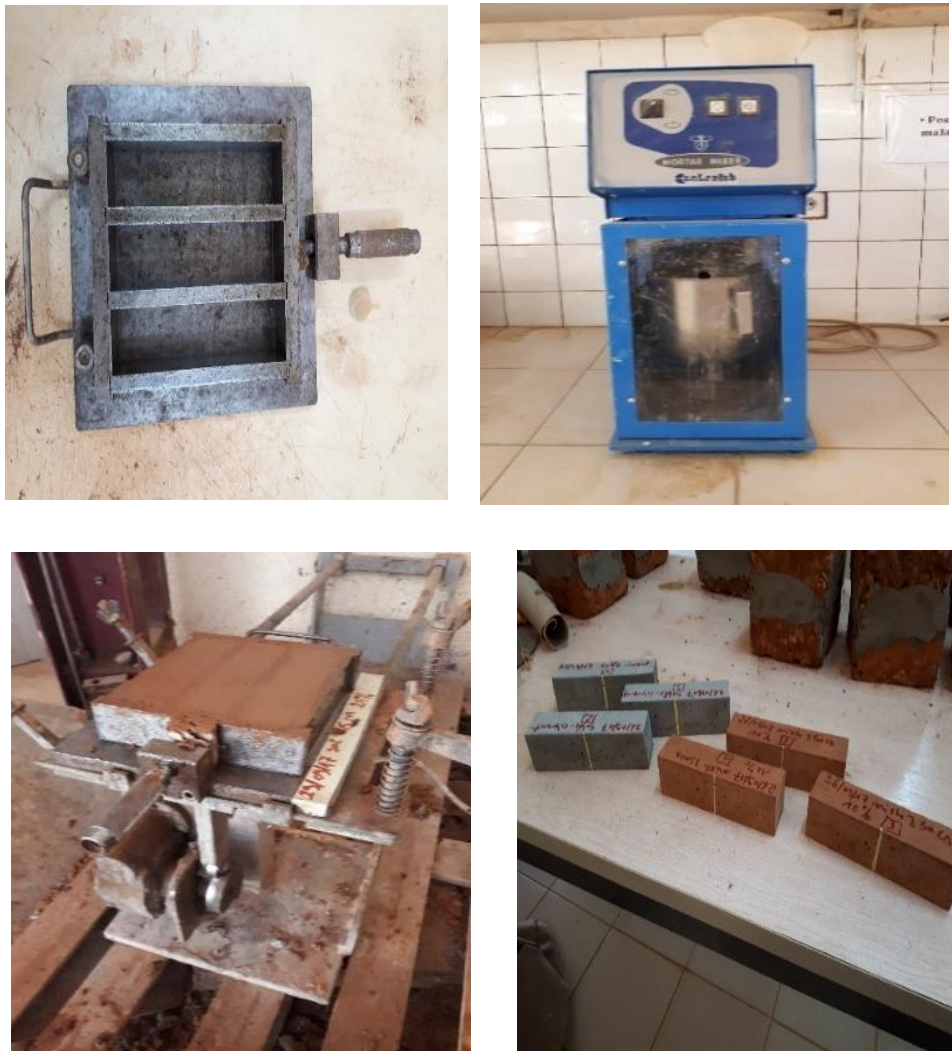
Photo 1 : Essai de compression parpaing
