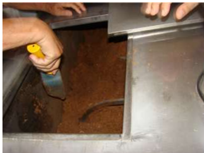
Figure A3-1b: Composting reactor of the commercial composting toilet (Saiwa Denko).
