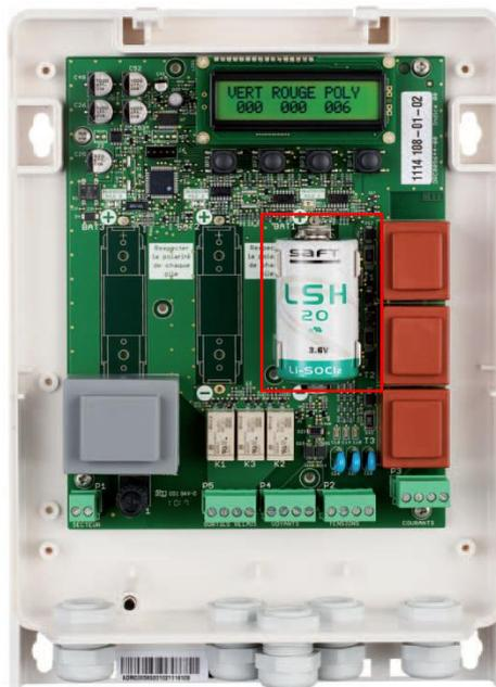
Figure 82: Alimentation autonome DAX
