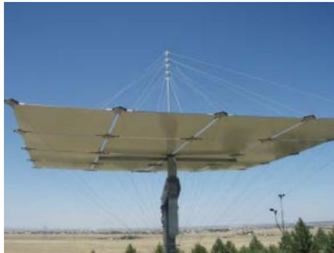
Figure 11. Héliostat Solaflect Energy [8]
