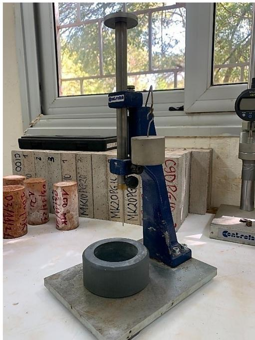
Figure 22: Appareil de Vicat manuel
