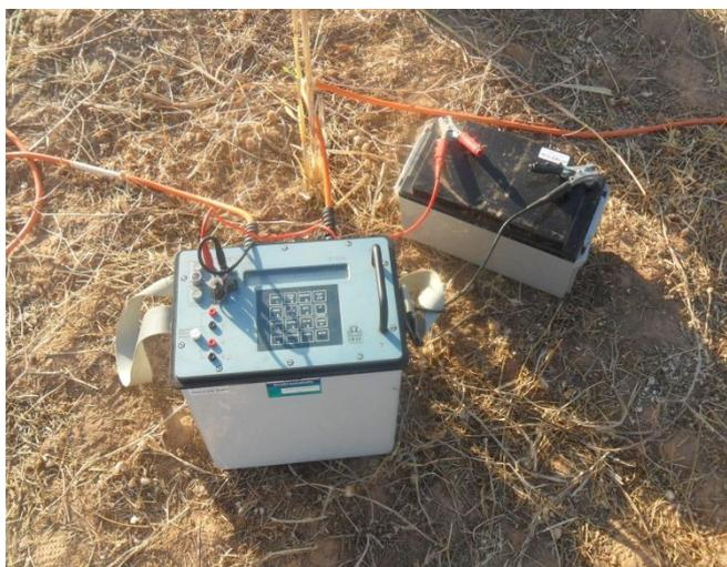
Figure 9: Syscal R1 plus 72 switches
