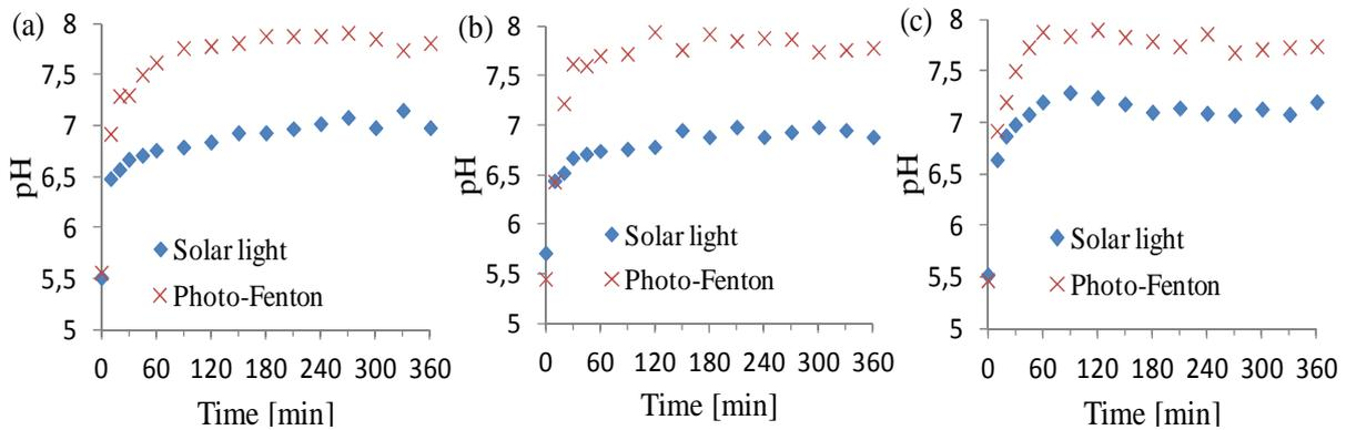
**Figure 3.5.** Variations of pH during the disinfection by solar light exposure and neutral photo-Fenton of total coliforms bacteria/*E. coli* and *Salmonella* spp. Recorded at different day time's intervals: (a) 8-14h, (b) 10-16h and (c) 12-18h.
