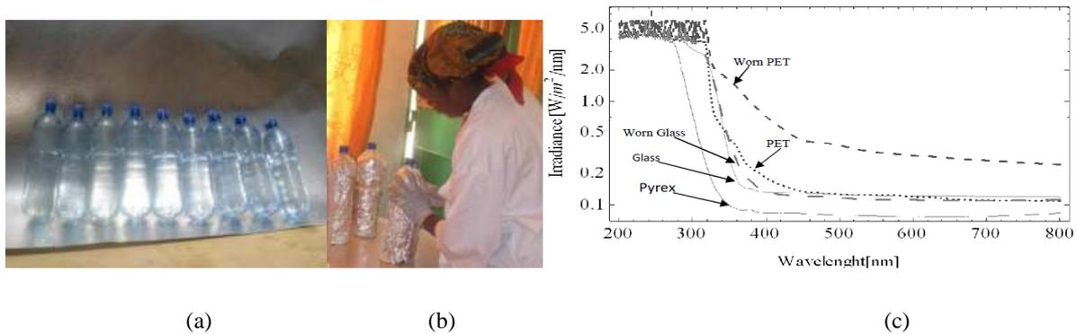
**Figure 2.1.** (a) 9 Pet bottles for the triplicate simultaneous exposure of the systems  $\text{H}_2\text{O}_2/\text{Fe}^{2+}/h\nu$ ,  $\text{H}_2\text{O}_2/h\nu$ , and  $h\nu$  (irradiation only). (b) Blank of each system, (c) Absorbance of different reactor materials (Pyrex, Glass, Pet).
