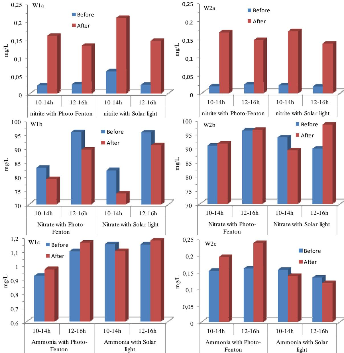
**Figure 5.4:** Evolution of nitrite (a), nitrate (b) and ammonia (c) concentration during the sole solar and photo-Fenton disinfection of two natural wells' water from Tanghin (W1) and Nonsin (W2) district of Ouagadougou. (Notice that the difference in the initial concentration of each chemical component in the results presented here are related to the fact that new water sample was collected and used for each new experiment).
