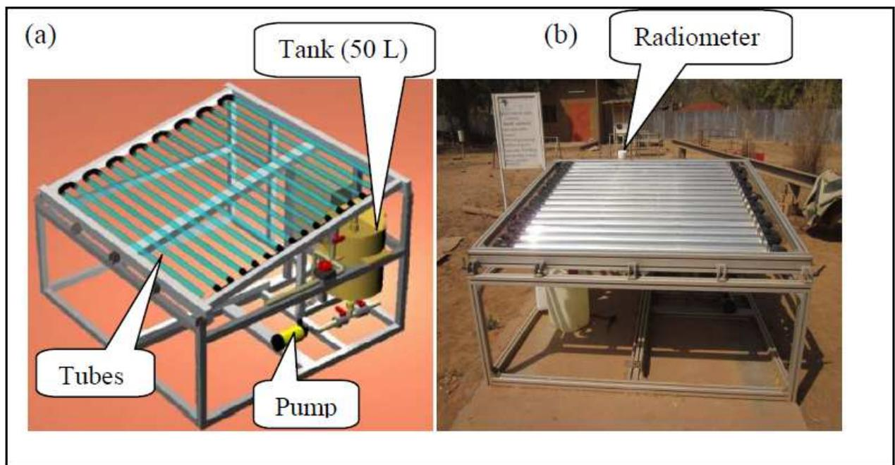
**Figure 3.1.** The schematic (a) and physical (b) representation of the compound parabolic collector (CPC) solar reactor.
