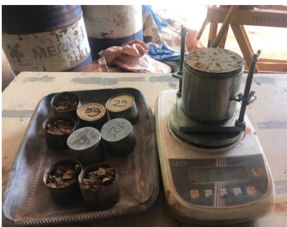
Image 5 : Essai proctor normal
