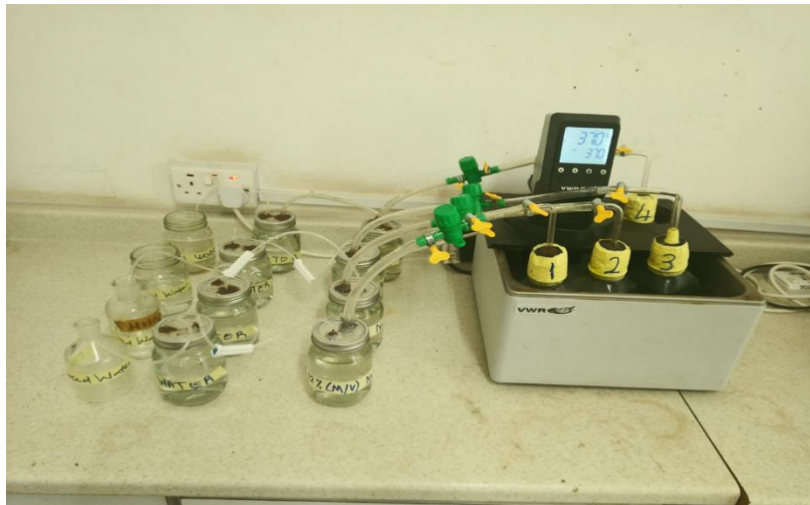
Figure 3-A: The SMA Test Experimental Setup
