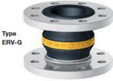
**YELLOW BAND** expansion joints suitable for petroleum based products with aromatic content up to 50 %, fuels (ethanol content up to 85 %), aviation fuels, town gas and natural gas except liquefied petroleum gas. Temperature range (depending on medium) -20°C up to +90°C, temporarily up to +100°C. Electrically dissipative.
