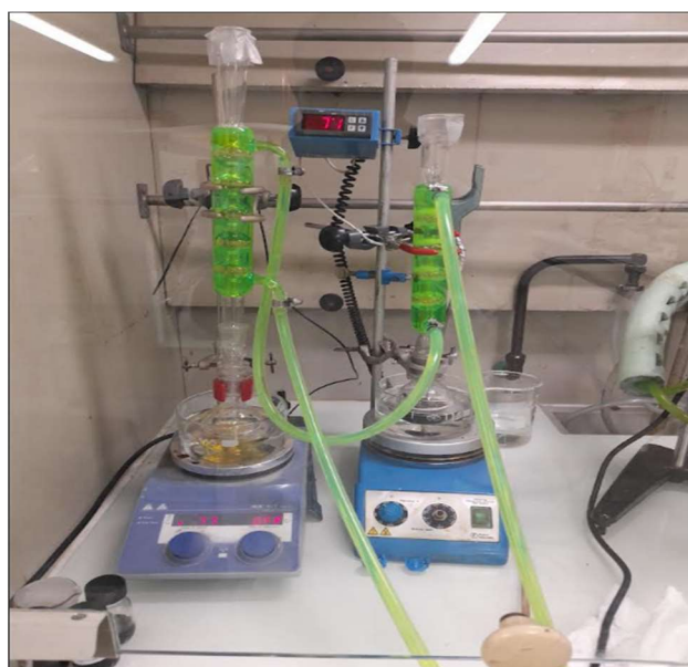
Figure 2.12. System used for accelerated ageing of fuel blends.
