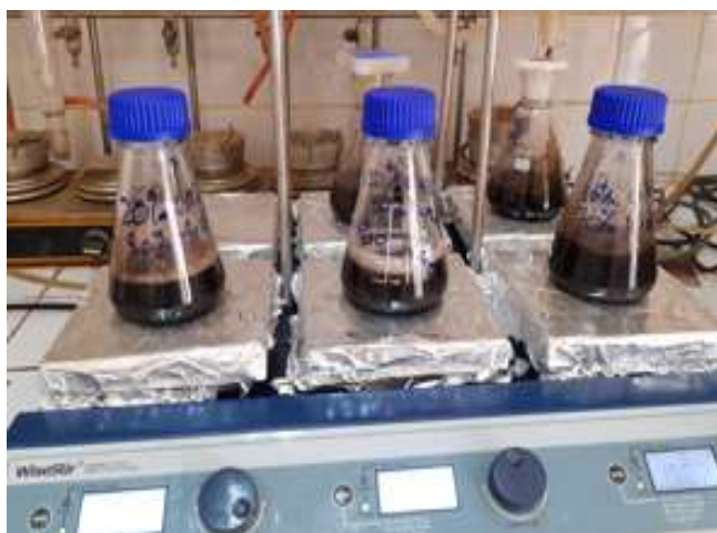
Figure 2.10. Preparation of fuel blends
