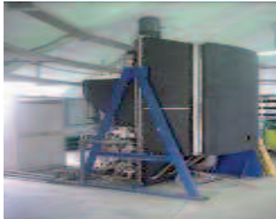
Figure 7. VVC desalination unit.
